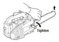
While lifting the chain guide, turn the content screw to apply correct tension to the chain. Then lock the crankcase nuts.
