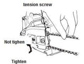
8) Tighten the nuts and check if the chain is rotated correctly and tight.
