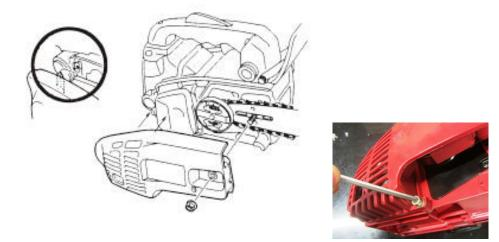
7) Adjust the chain tension by turning the tension screw until the straps touch just the bottom side of the bar.
